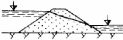
Figure 2.1 Homogeneous embankment dam [Goldin and Rasskazov, 1992]
