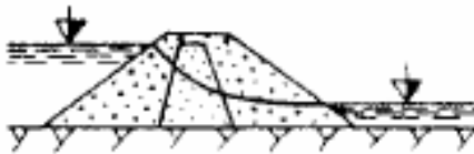
Figure 2.2 Zoned embankment dam with thin central core [Goldin and Rasskazov, 1992]
